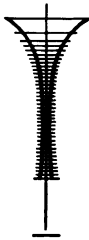
FIG. 123.— Wulsty Castle : Turbine Blade Ring Showing Proportioning to Meet Increase in Steam Volume
